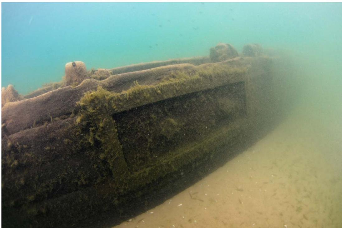
Figure 7. Starboard side lumber port aft of foremast chain plates, looking forward.
