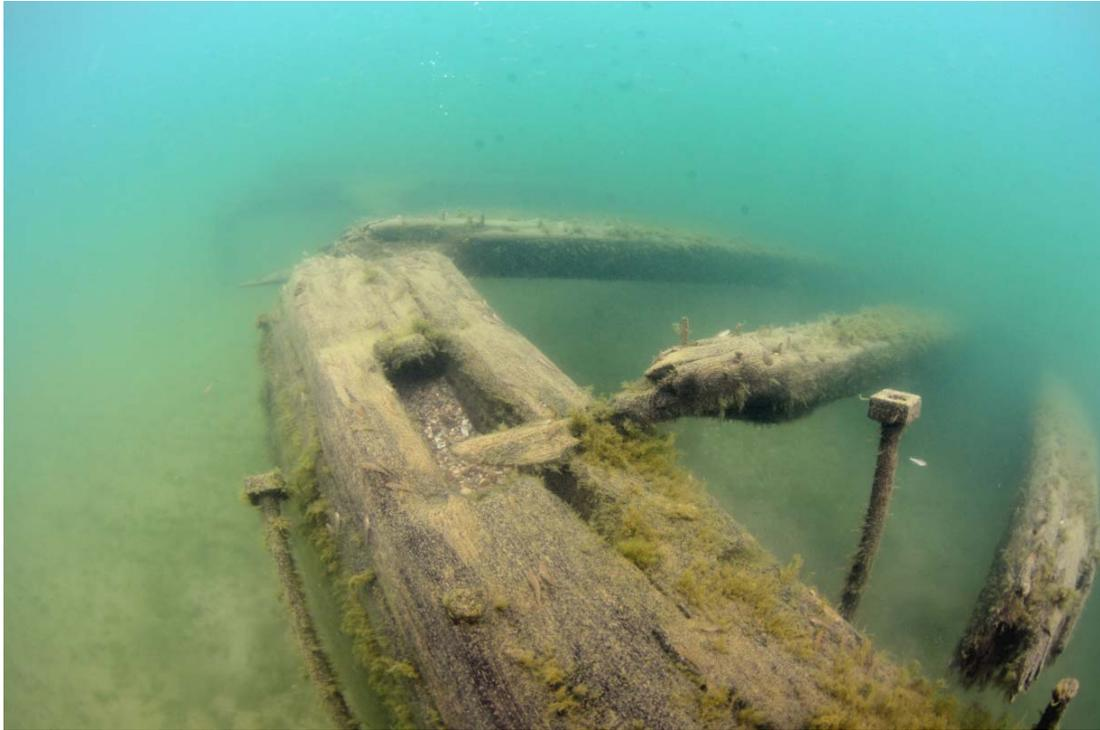
Figure 8. Aft end of the centerboard trunk with port side deck beams, looking aft.
