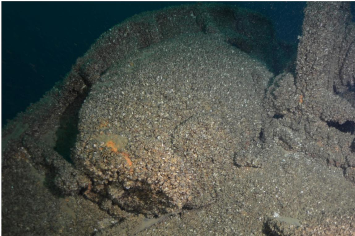
Figure 60. Spare propeller blade along the bulwark on the stern.
