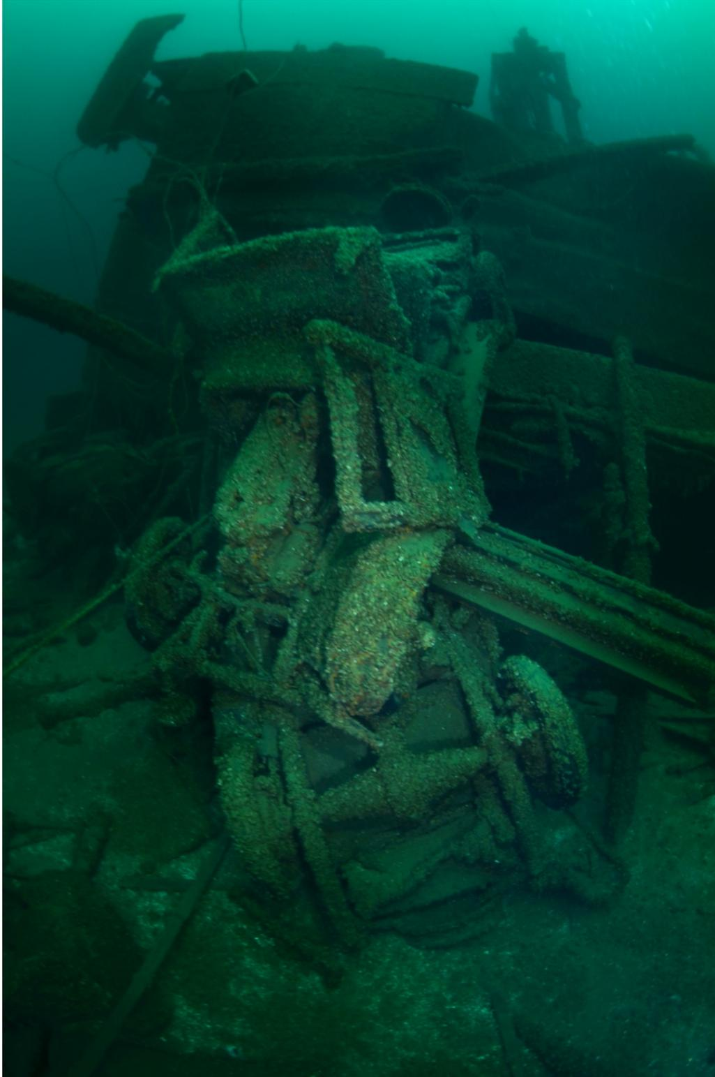
Figure 47. Car #4 (a 2-door Nash sedan, on top) and Car #5 (a 4-door Nash sedan, bottom) spilling out of the break at the aft end of the bow section.
