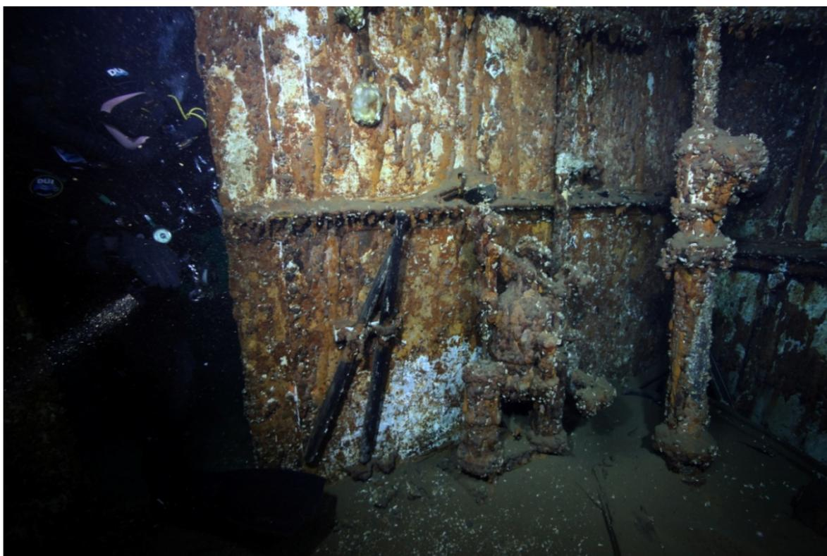
Figure 36. Double acting bilge pump with handles, forward of the bulkhead in the windlass room. Photo courtesy of John Janzen.
