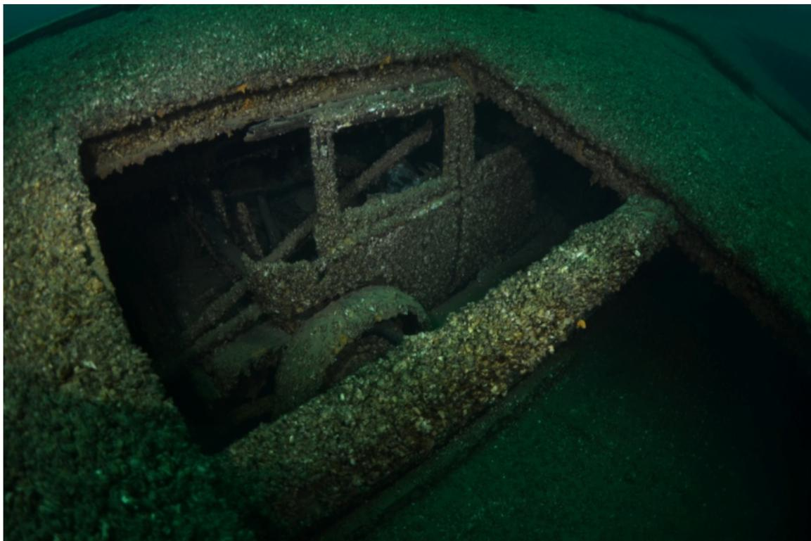
Figure 48. Car #7 a Nash 2-door closed body design, as viewed through grain hatch #1.
