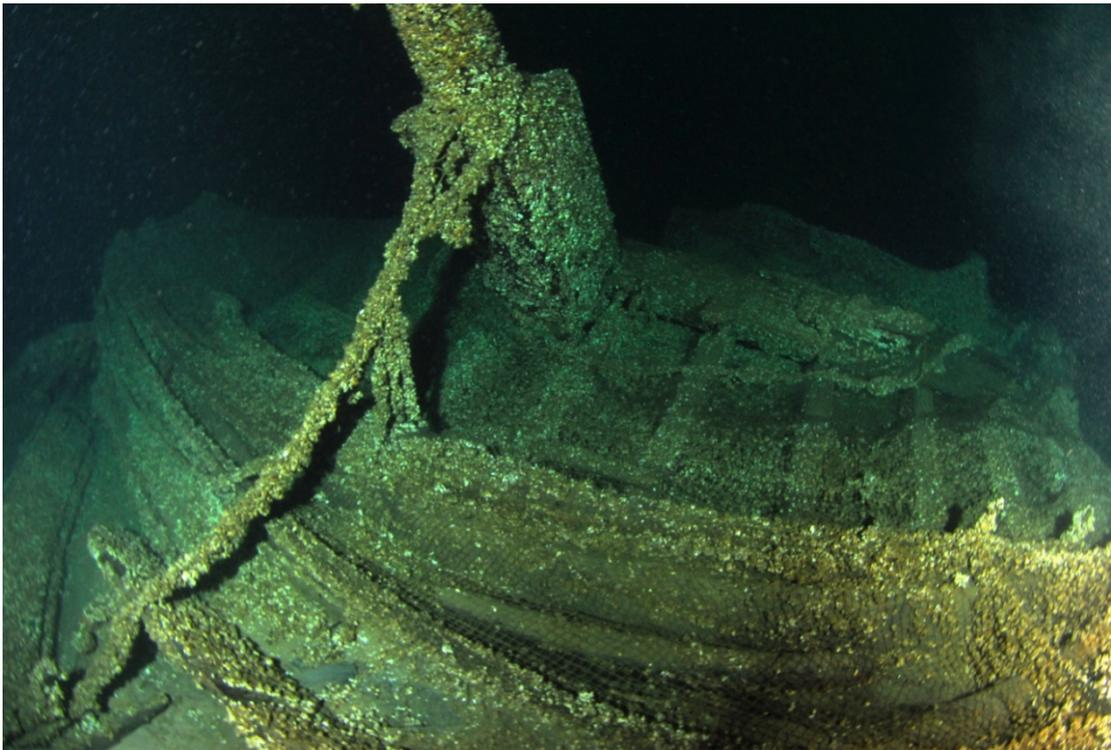
Figure 14. Rudder box and transom of the *Floretta* fallen aft and covered by fishing nets. Photo courtesy of Pete Nawrocky.
