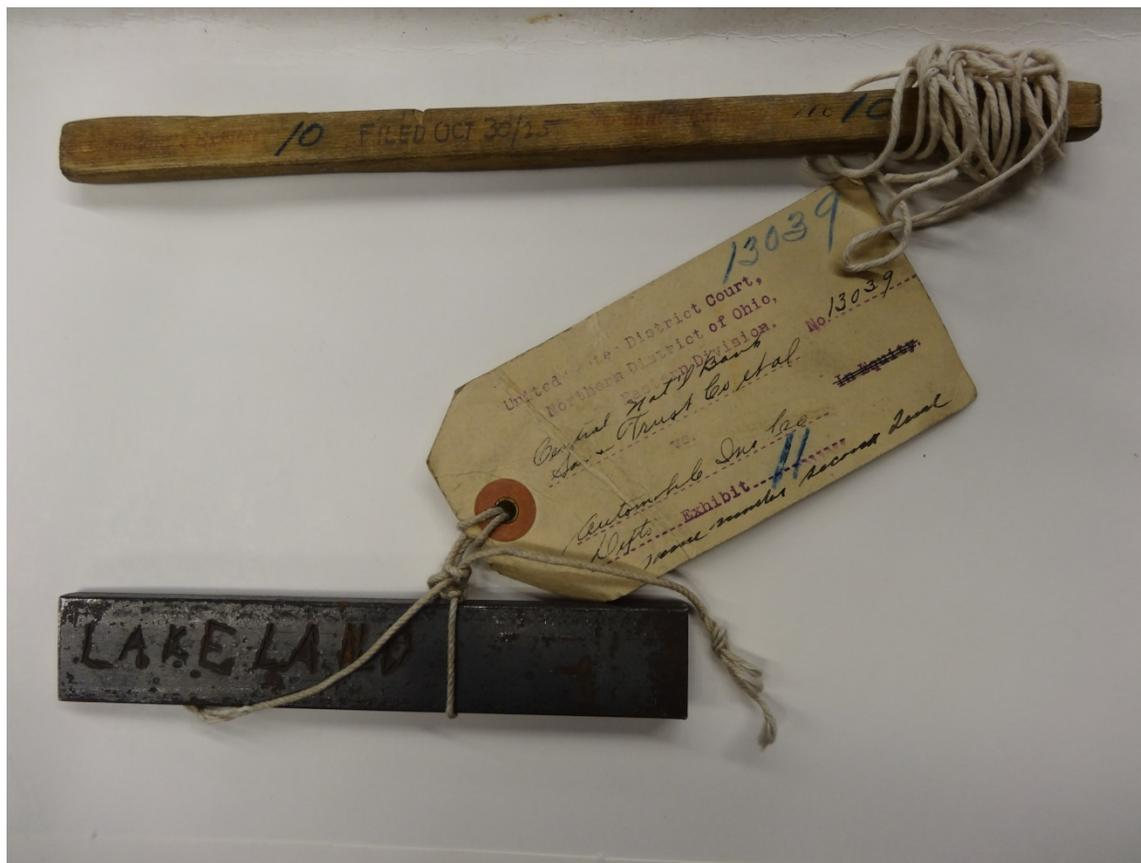
Figure 31. Wood stick and steel blank used to measure the open sea-cock valve on the *Lakeland*.
