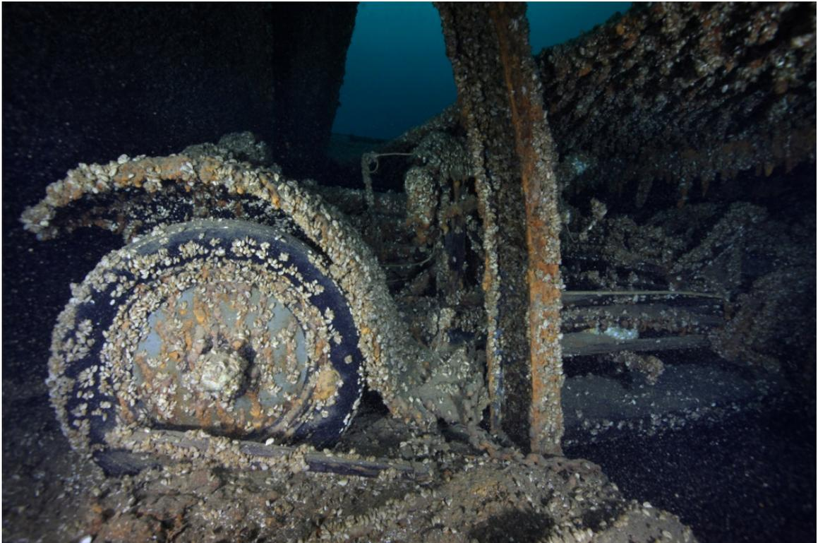
Figure 46. Car #6, a Nash Victoria coupe or 2-door sedan, with overhead valve engine and disk wheels. Photo courtesy of John Janzen.
